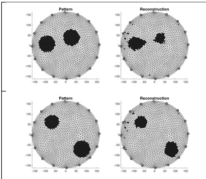
Fig 2. Patterns and reconstructions for the system with 16 measured sensors.
