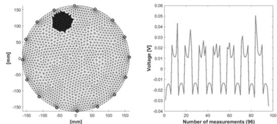
Fig. 1. An example of simulation of imaging domain with a graph showing the voltage measurements.
