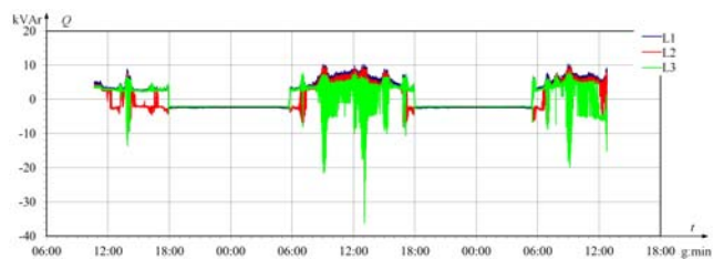
Fig. 12. Variations of reactive power value of the fundamental harmonic generated within three days by the PV power station
