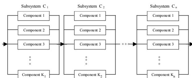
Fig. 1. Series-parallel power system structure
