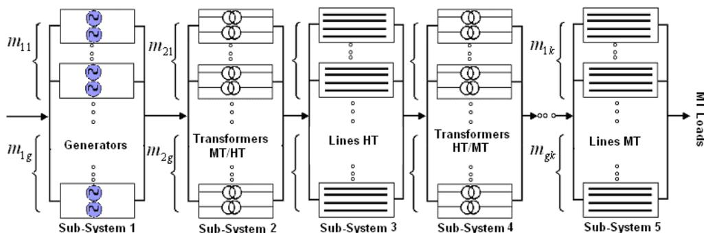
Fig. 8.1. Series- parallel power design
