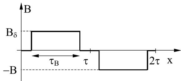
Fig.4. Radial magnetization in the slot
