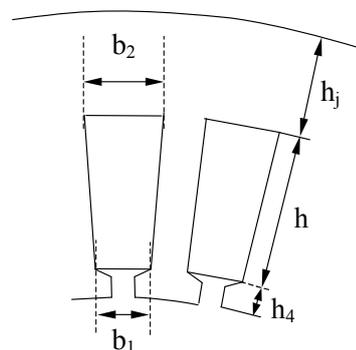
Fig. 2. Machine dimensions and graphic definition of argument h.
