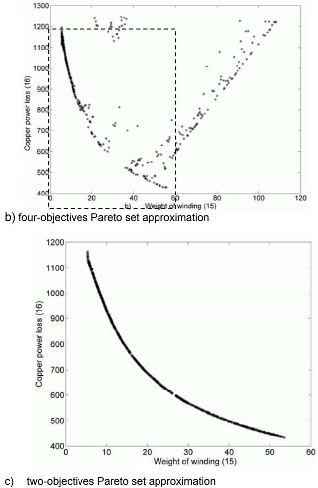
Fig.6 The weight winding (15) - copper power loss (16) for the Pareto sets approximations for a) five-, b) four-, c) two-objectives respectively. Please note the change of scale. The c) is enlargement of the dashed rectangles in a) and b). Number of points (solutions) is constant
