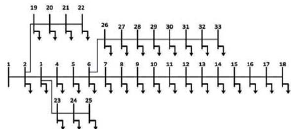
Fig.1. IEEE 33 bus test network
