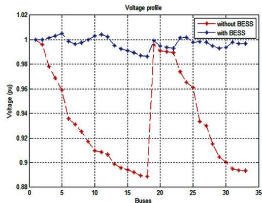
Fig.7. Voltage profile with and without integrated BESSs
