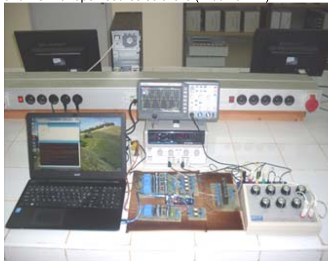
Fig.10. A Laboratory prototype of a Five-level inverter
