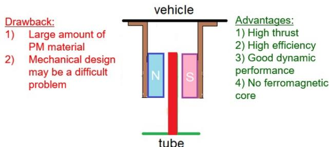
Fig. 16. Double-sided PM LSM with coreless primary (armature)
