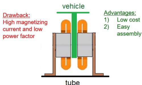
Fig. 15. Double-side LIM with aluminum secondary (reaction rail)
