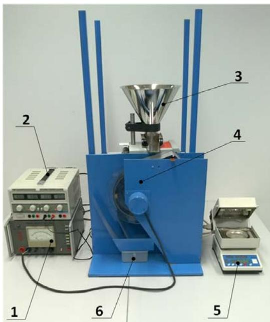
Fig. 1. Test stand: 1 - HV power supply, 2 - DC power supply for drum drive, 3 - material feeder, 4 - electroseparator with bifilar winding, 5 - moisture analyser, 6 - divisible container for 2 chambers
