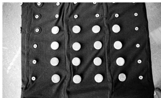
Fig. 4. Diagrams of building silicone electrodes with their placement on the vest.
