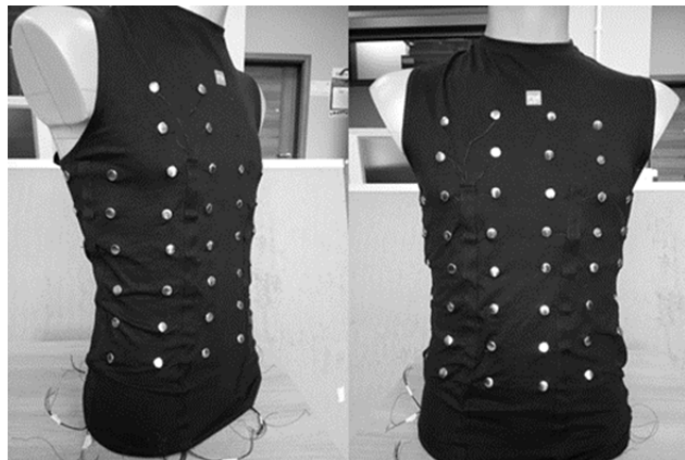
Fig. 2. Vest with wiring and visible rivets.
