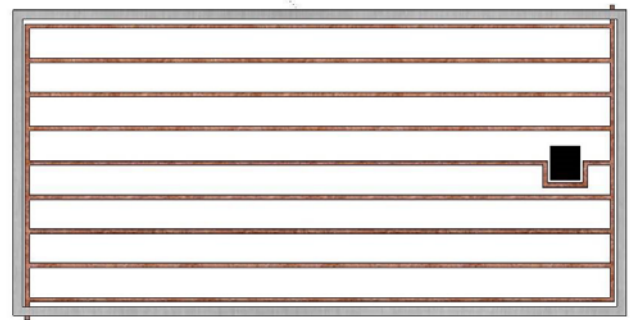
Fig.3. Sheet-and-tube collector mounted on the backside of the PV module.
