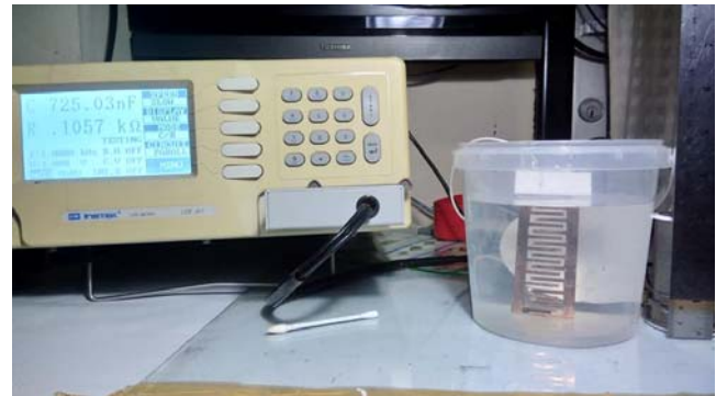
Fig.4. The measurement setup for IDC level sensor.
