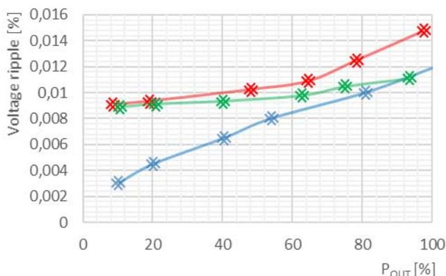
Fig.7. Output voltage ripple in dependency on output power change for three different values of input voltage (red – 14V, blue – 12V, green – 9V)
