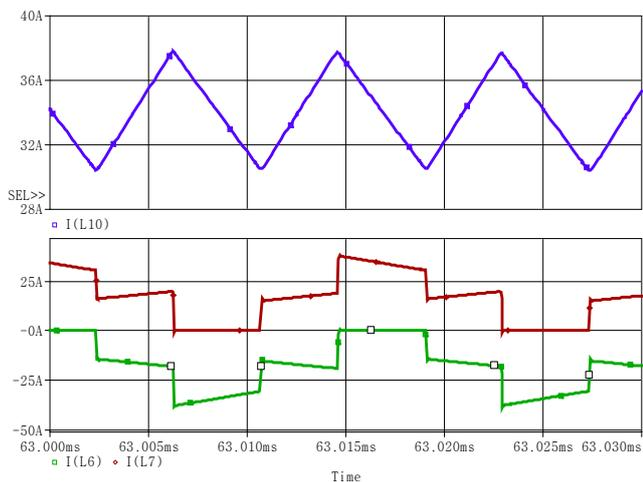
Fig.4. Waveforms of boost inductor current (blue), and primary transformer coils currents (red and green)
