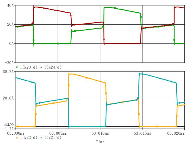
Fig.5. Waveforms switching transistors for converter A (red and green) and waveforms switching transistors for converter B (yellow and grey)
