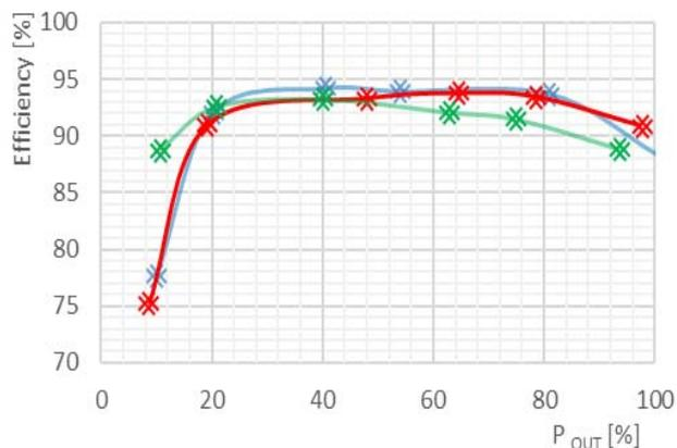
Fig.6. Efficiency in dependency on output power change for three different values of input voltage (red – 14V, blue – 12V, green – 9V)
