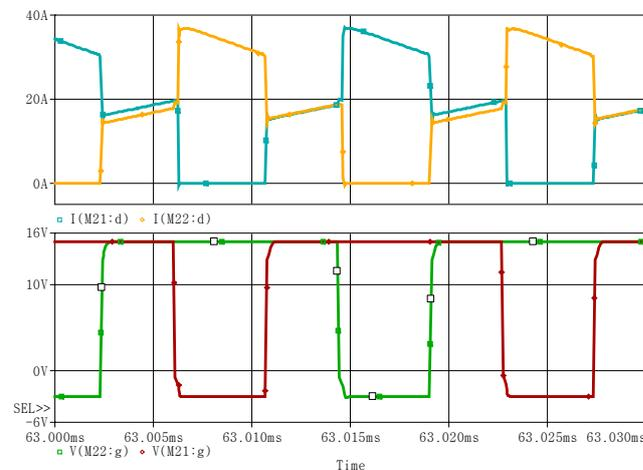
Fig.3. Waveforms switching transistors currents (yellow and grey), and switching transistors gate signals (red and green)
