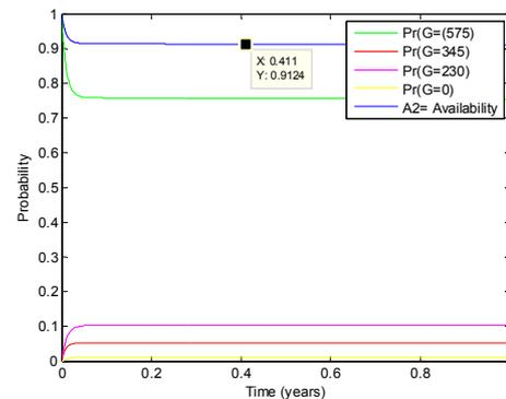
Fig.4. Availability and probabilities of different levels of performance for  $w=230 \text{ kV}$
