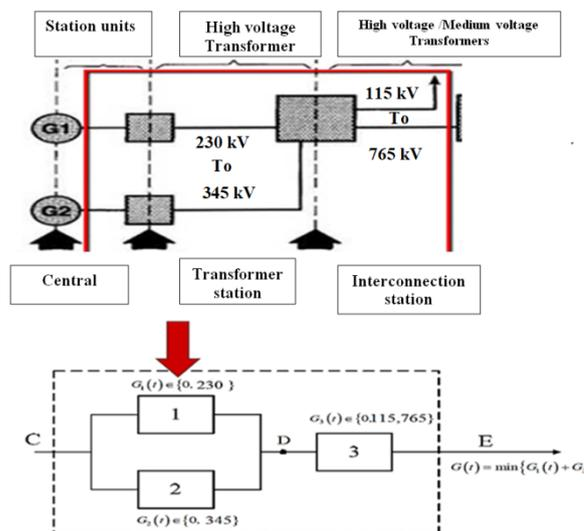
Fig.2. A multi-state system with 3 elements (Transformers).
