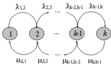
Fig.1. Markov Model Diagram of Repairable MSS Component
