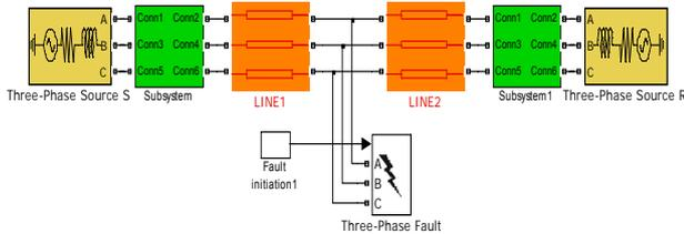
Fig. 5: Matlab / Simulink view of transmission line.
