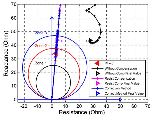
Fig. 7: Fault applied at 108 km from relay location (in zone 2)
