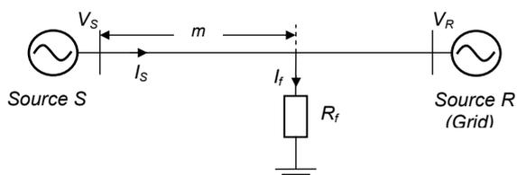
Fig. 4: Fault in transmission line at a distance  $m$ .
