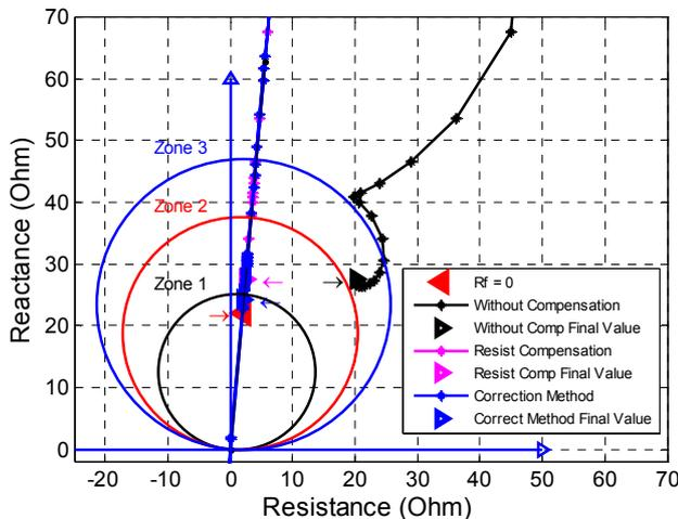
Fig. 6: Fault applied at 70 km from relay location (in zone 1)
