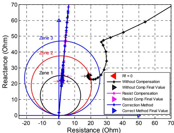
Fig. 9: Fault applied at 70 km from relay location (in zone 1)
