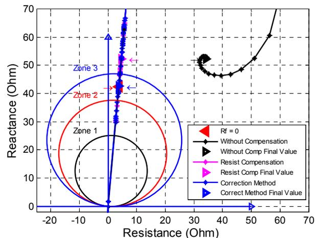
Fig. 11: Fault applied at 135 km from relay location (in zone 3)
