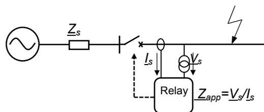
Fig. 1: Mho distance relay principle.
