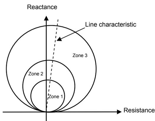
Fig 2: Mho Relay characteristic.
