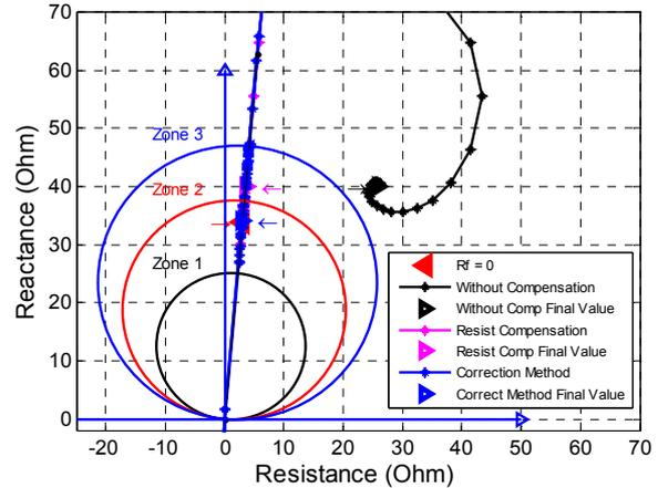
Fig. 10: Fault applied at 108 km from relay location (in zone 2)
