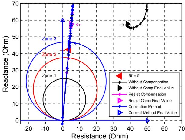
Fig. 8: Fault applied at 135 km from relay location (in zone 3).
