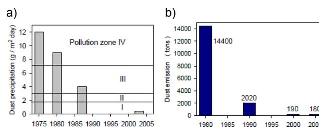
Fig.1. Dust deposit density at test station (a), dust emission of Glogow Smelting Plant (b), [4]
