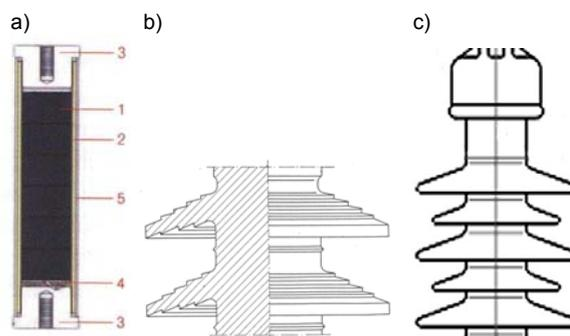
Fig.10. Cross section of surge arrester ASW18 (a), 1-varistor column, 2-glass-epoxy pipe, 3-electrodes, 4-spring washer, 5-silicone housing [29], Insulator with stepped sheds LPZS75/15 (b) [30], porcelain insulator LP75/27W with alternating sheds (c)
