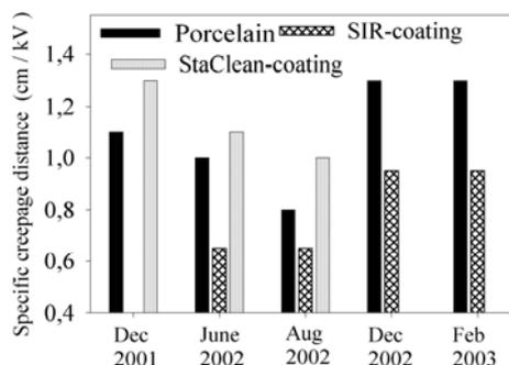
Fig. 6. Flow on test results (spray wetting of natural pollution). The specific withstand leakage distance of post SWZP with bare glaze (porcelain), with silicone coating (SIR) and with fluorourethane coating (StaClean coating).
