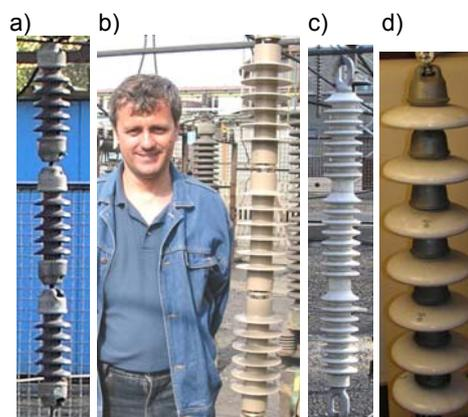
Fig.7. Insulators with the special hydrophobic glazes (a), insulators with hydrophobic epoxy resin (b), Insulators made of polymer concrete (c), cap and pin insulators with semi conductive glazes (d)
