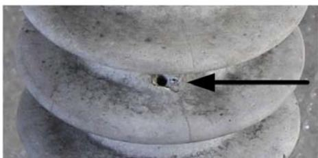
Fig.8. Breakdown channel through polymer concrete
