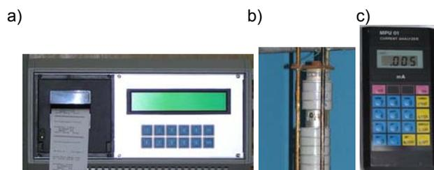
Fig.5. Leakage Current Monitor LCM (a), TINYTALK temperature probe mounted in a ZnO varistor column (b), current analyser MPU 01 (c).
