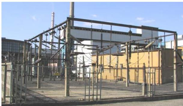
Fig.2. Insulator field, the small (yellow) building contained a 6 kV substation and the command room, the white cubic room housed the pollution chamber.
