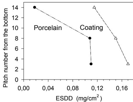
Fig.11. ESDD on the LP75/27W long-rod insulator with the SIR coating or on the insulator with the bare glazes. Measurements on smaller sheds below the greater sheds in May 2006 [32]
