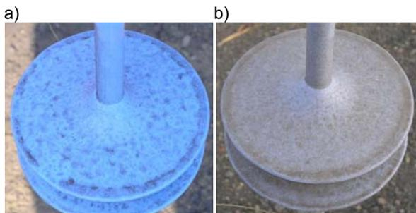
Fig.12. Colour change of the silicone rubber insulators with exposition time at Glogow Pollution Test Station. a – after one month, b – after 8 months
