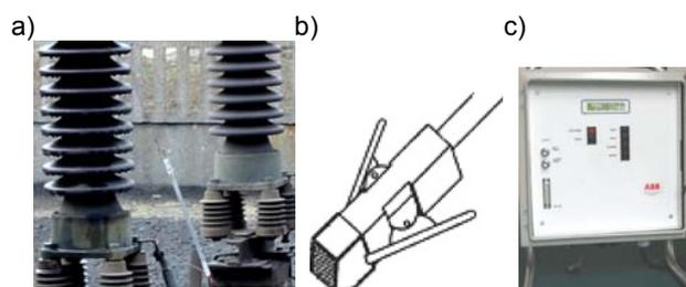
Fig.4. SWZP post insulator with 8 sheds short circuited by the fuse indicator of the pollution flashover (a), strip probe for surface conductivity measurement (b), Current Pulse Integrator CPI (c).
