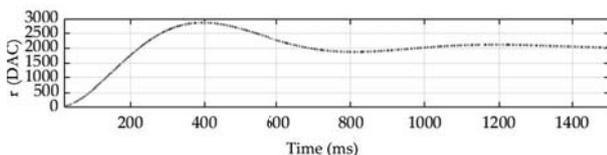
Fig. 6. Closed loop response of  $r$  in the HIL simulation.
