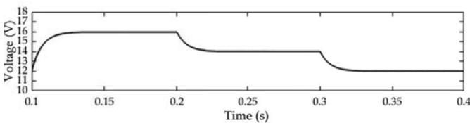
Fig. 13. Capacitor output voltage for SFL control of SEPIC converter - Matlab simulation
