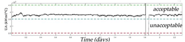
Fig. 10. Global coefficient x Area (UA) of the exchanger estimated in HIL
