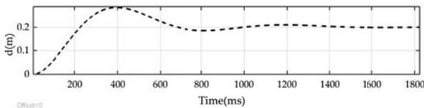
Fig. 5. Closed loop response of  $r$  in a conventional Matlab simulation.
