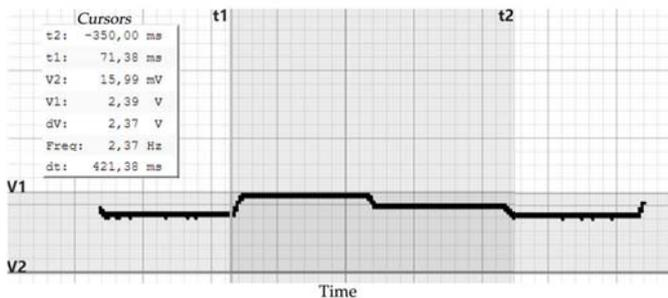
Fig. 14. Capacitor output voltage for the SFL control of the SEPIC converter - HIL simulation. Note: 0.1 s / div on the x axis; on the y axis a 2.4 V in DA converter corresponds to 16V of the real voltage.
