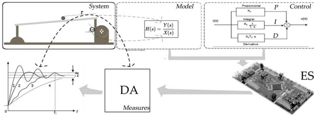
Fig. 4. Ball and Beam HIL simulation
