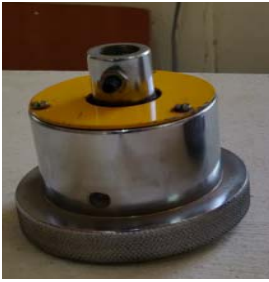
Fig 4: Rigid support of tail stock
