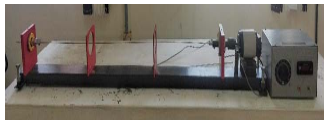
Fig 3: Whirling of shaft
