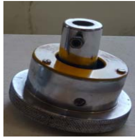
Fig 5: Flexible support of tail stock
