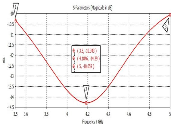
Fig. 2. Return loss performances of the proposed antenna.
