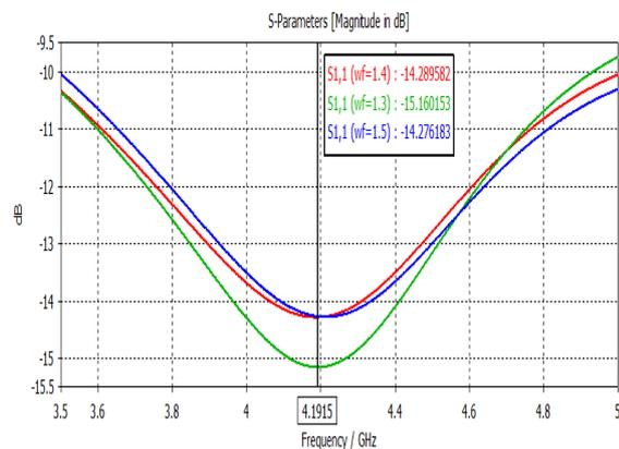
Fig. 3. Comparison of return loss performances based on the width of the feedline.
