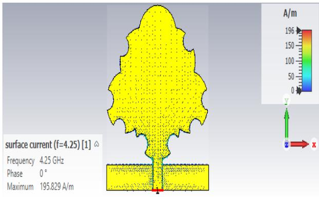
Fig. 5. Current distribution of the intended at 4.25 GHz.
