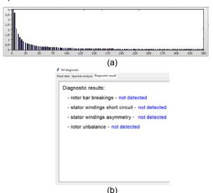
Fig. 5 Diagnostic for IM without breakings
