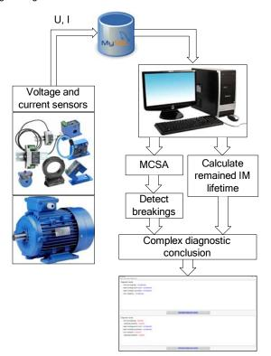
Fig. 4 Diagnosis system schema
