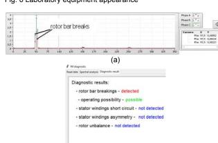
(b) Fig. 7 Diagnostic for IM with the broken rotor bar
