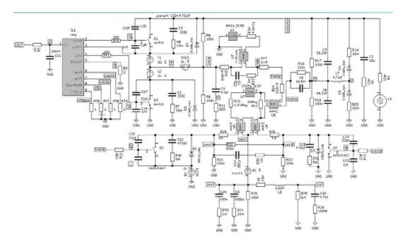
Fig.2. Schematic of the simulated system with measured values of inductances and parasitic elements of real LLC resonant circuit.
