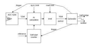
Fig. 3. Output voltage controller block diagram
