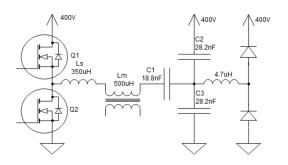
Fig.1. Overview of the components in the LLC resonant converter with quality factor limiter [5]
