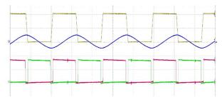
Fig. 6. Converter measurements for 100mA output load (5 us/div).Yellow: half-bridge voltage (200 V/div); blue: Ls current (2 A/div); pink and green: half-bridge driving signals (2 V/div).
