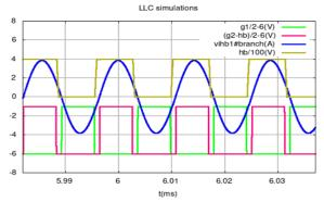
Fig. 9. Converter simulations for 30 A output load.
