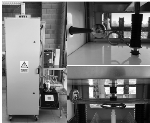
Fig.2. View of the test stand together with the method of test object assembly
