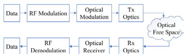
Fig.1. Basic Architecture of a Radio over Free Space Optical Communication System
