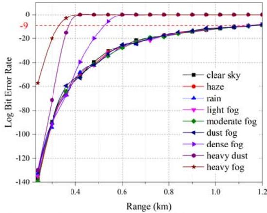
Fig.3. Range vs. Bit Error Rate of the RoFSO Link
