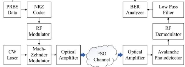
Fig.2. Simulation Setup of the Radio over Free Space Optical Communication Link
