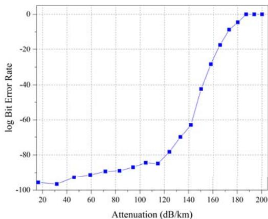
Fig.5. Attenuation vs. Bit Error Rate Performance of the RoFSO Link for a Range of 300 meters
