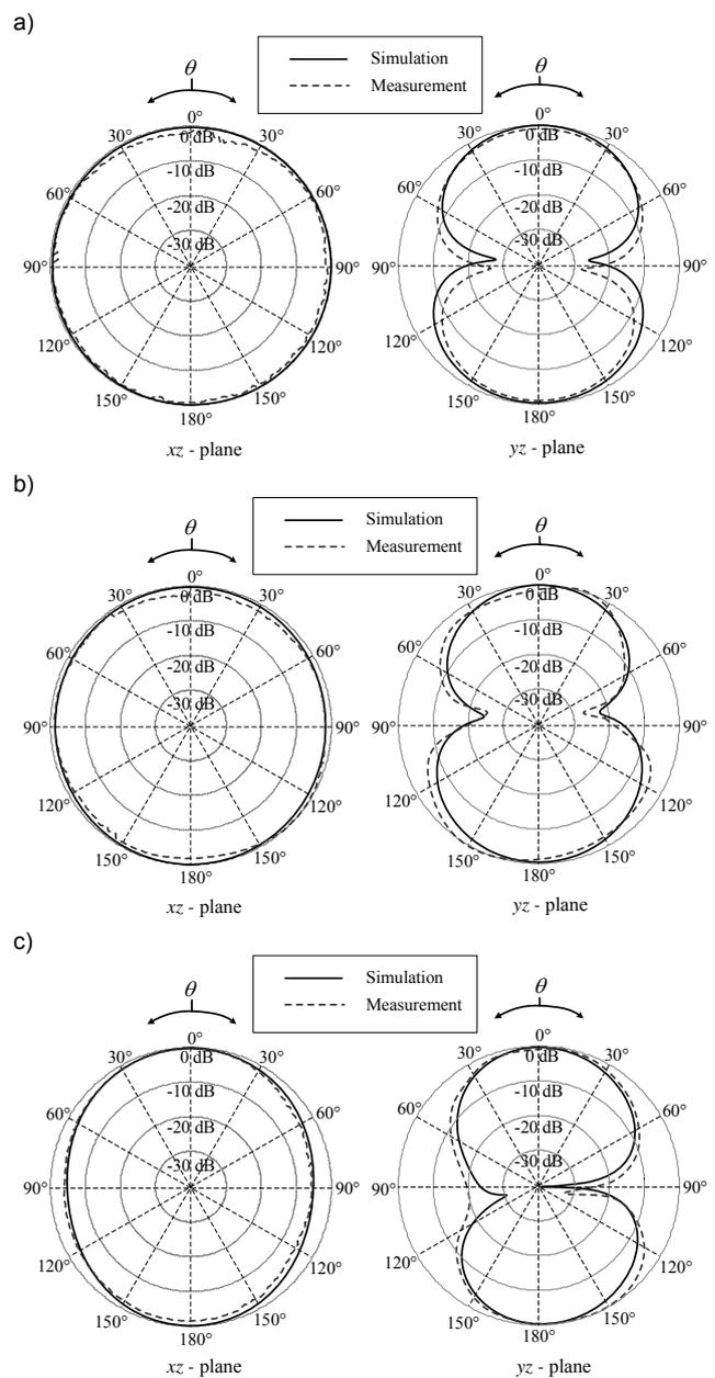
Fig.7. Radiation pattern in xz- and yz-planes at: a) 2.45 GHz, b) 3.5 GHz and c) 5.5 GHz
