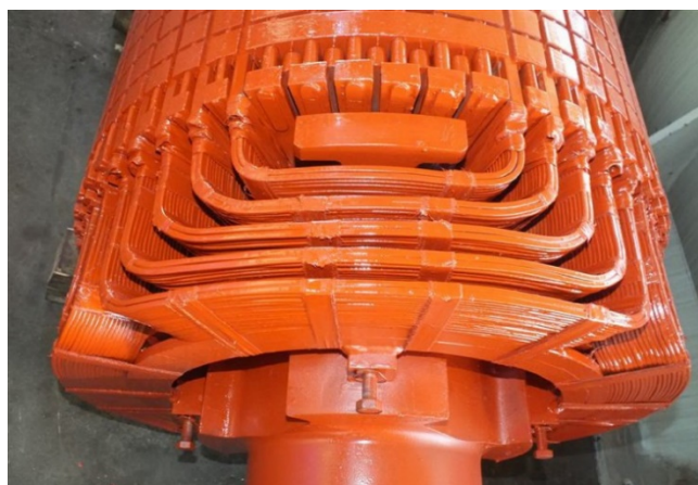
Fig. 1. The end windings of the excitation winding and start-up cage winding of asynchronous motor, rated at: 7400 kW, 6 kV- Y. 814 A, rotor - 180 V DC, 335 A, 1500 rpm
