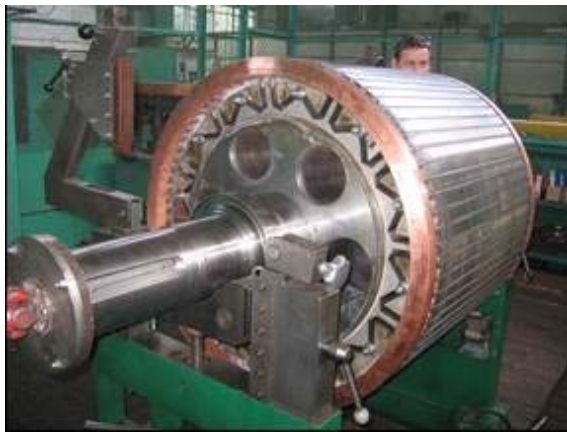
Fig. 3. Rotor of synchronous motor (LSPMSM) with permanent magnets and cage start-up winding; motor rated at 1100 kW, 6 kV, 500 rpm [8]
