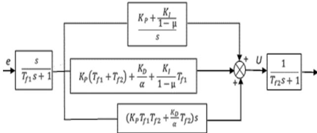
Fig. 4. Block diagram of the fractional order PID-regulator.
