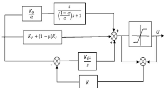
Fig. 6. Block diagram of the PID- controller with „anti wind-up” block.
