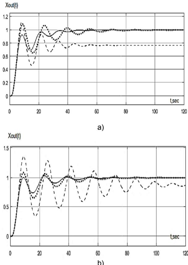
Fig. 7. Transients of the different type of PID-controller (— - fractional PID-regulator according to the scheme of fig. 1; - - - - classic PID- controller; ..... - fractional PID-controller according to the scheme of fig. 2) and for two cases (a - when  $\mu=0.6$ , b - when  $\mu=0.9$ )
