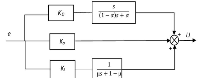
Fig.2. Block diagram of the fractional order PID-controller obtained using an integrated operator with a non-singular core [20].
