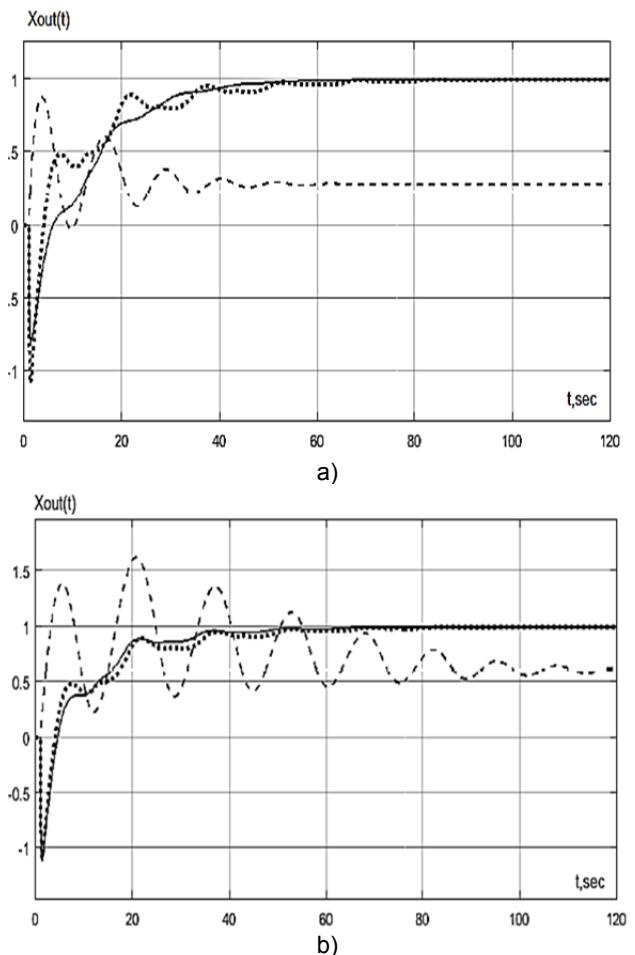
Fig. 8. Transients of the different type of PID-controller and by block of signal limitation (— - fractional PID- controller according to the scheme of fig. 1; - - - - classic PID- controller; ..... - fractional PID-regulator according to the scheme of fig. 2.) and for two cases (a - when  $\mu=0.6$ , b - when  $\mu=0.9$ )
