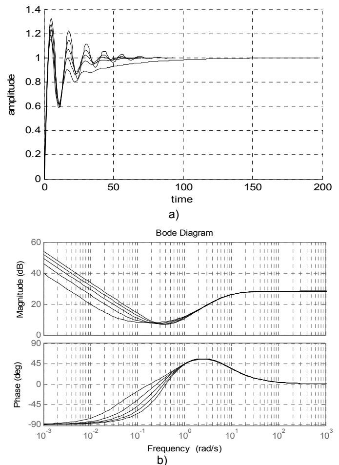
Fig. 3. Effect of parameter  $\mu$  changing on transient characteristic of system and frequency characteristics in case of the fractional controller
