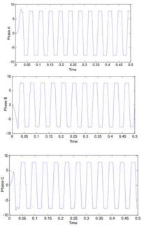
Fig.7 Electromagnetic force variation for phase a, b and c respectively.
