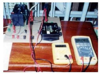
Fig. 15. An electrical system connection for testing the impressed current corrosion protection of the metal pipes.
