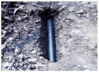
Fig. 13. The metal pipe used for the impressed current corrosion protection test.
