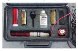
Fig. 16. The Cu/CuSo 4 probe for measuring the anti-corrosion performance of the metal pipes.
