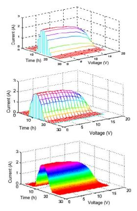
Fig. 5. The results of the three-dimensional surface shape values in various ways from the solar panel test data.
