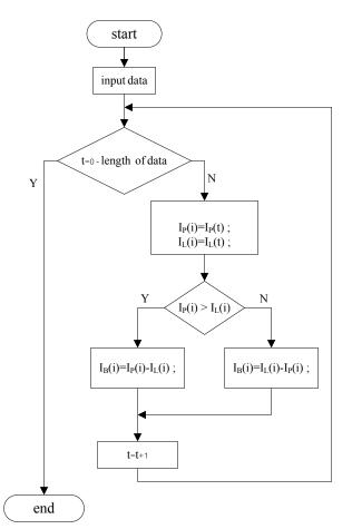
Fig. 4. Steps for calculating the current values at each section of the solar power system.
