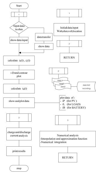
Fig. 2. Workflow of the simulator and analyzing the solar power system.
