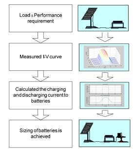
Fig. 3. Order of each part of the procedure for analyzing the solar power systems according to the proposed method.
