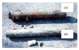
Fig. 17. Results of the structural comparison of the non-corrosionprotected pipes (A) with the impressed current corrosion protection metal pipes (B).
