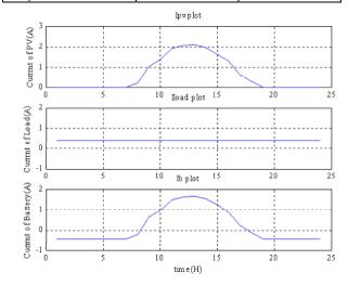
Fig. 9. Hourly diagrams of the load currents and battery currents 24 hours/day.
