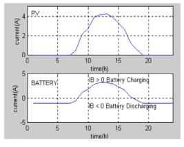
Fig. 7. The results of showing the current values at each time of the solar power system.
