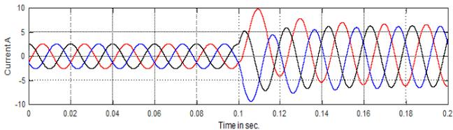
Fig.14. Secondary current at external fault
