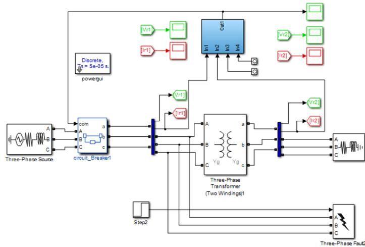
Fig.6. Modeling circuit of differential relay protection
