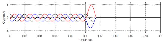
Fig.19. Current at line-to-line fault
