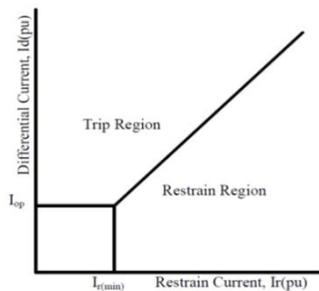
Fig.3. Differential relay characteristics.
