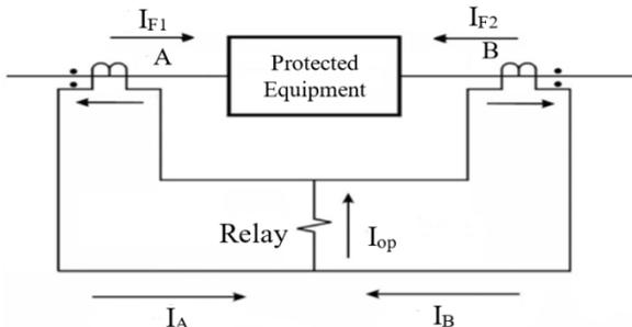
Fig.2. Equivalent circuit of differential relay for single phase.
