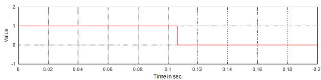
Fig.15. Differential relay output signal
