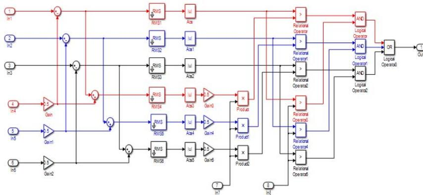
Fig.7. Scheme of differential relay subsystem
