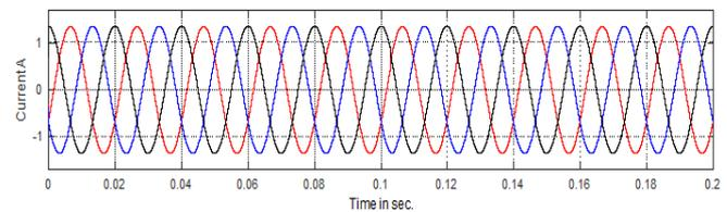
Fig.9. Primary current at no fault
