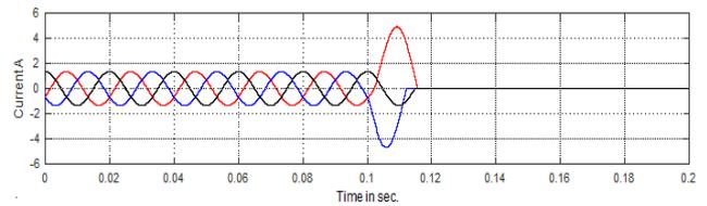
Fig.17. Current at line-to-line-to-ground fault
