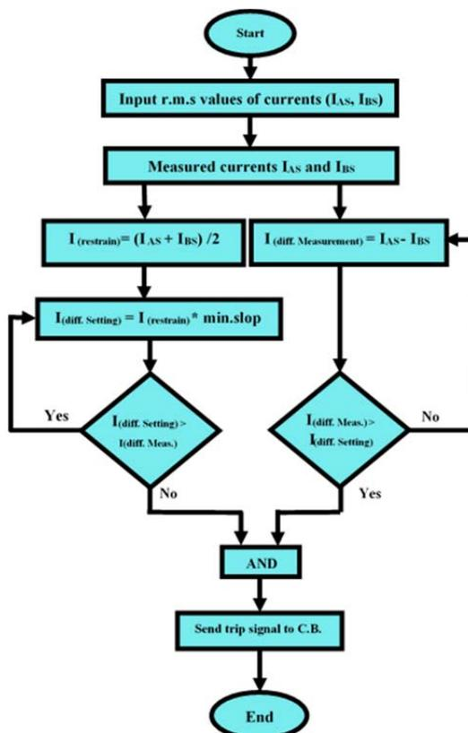
Fig.4. Flowchart of the differential relay for single line.
