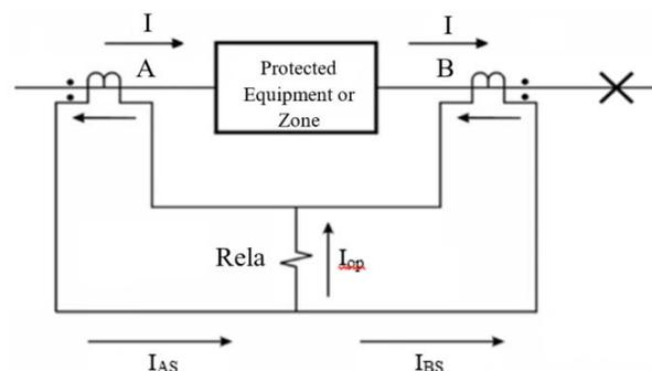
Fig.1. Differentials relay current at the time for out of zone.
