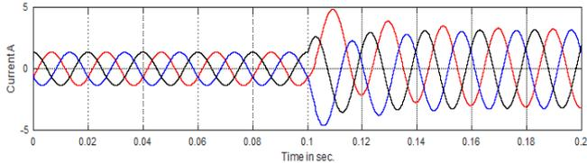
Fig.13. Primary current at external fault
