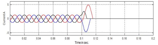
Fig.18. Current at three phase-to-ground fault
