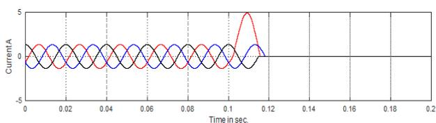
Fig.16. Current at line-to-ground fault
