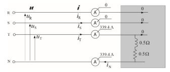
Fig. 2. An example of an unbalanced load.
