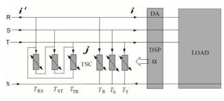
Fig. 9. A structure of an adaptive compensator.
