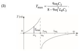
Fig. 11. Change of the TCS branch in the thyristor OFF state.
