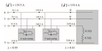
Fig. 13. The load with the adaptive compensator.
