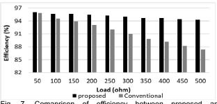
Fig. 7. Comaprison of efficiency between proposed and conventional converter for load variation (Fs=5 kHz, D=0.5)
