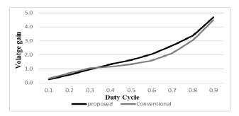
Fig. 6. Comaprison of voltage gain between proposed & conventional converter for duty cycle variation (Ro=100 $\Omega$ , Fs=5kHz)
