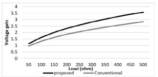
Fig. 8. Comaprison of volatge gain between proposed and conventional converter for load variation (Fs=5 kHz, D=0.5)
