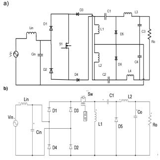
Fig.1. Proposed Single-Phase AC-DC Zeta Converter (a), Conventional Single-Phase AC-DC Zeta Converter (b)
