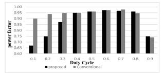
Fig. 4. Comaprison of input PF between proposed and conventional converter for duty cycle variation (Ro=100 $\Omega$ , Fs=5 kHz)
