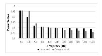
Fig. 9. Comparison of power factor between proposed & conventional converter under Fs variation (D=0.5 and Ro=100 $\Omega$ )
