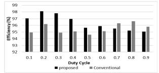
Fig. 5. Comaprison of efficiency between proposed & conventional converter for duty cycle variation (Ro=100 $\Omega$ , Fs=5 kHz)
