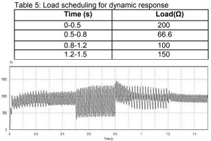
Fig. 15. Waveform of output voltage for dynamic response
