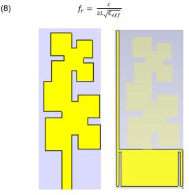
Fig.1: A Fractal Sierpinski single antenna
