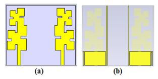
Fig.4: Fractal MIMO antenna (a) Patch plane (b) Ground plane
