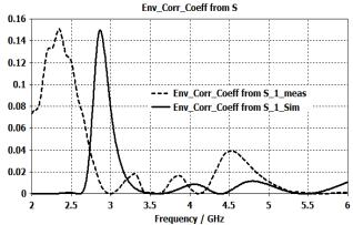
Fig. 14: Simulated and Measured ECC of the Fractal MIMO Antenna
