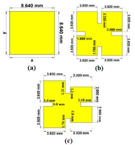
Fig.3: configration of fractal antenna (a) inatiator antenna , (b)  $0^{\text{th}}$  iteration (c) modified patch
