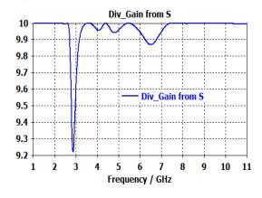
Fig. 8: DG of Disc MIMO Antenna
