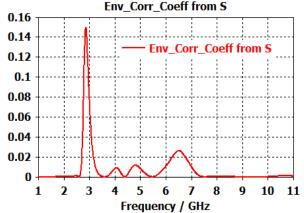
Fig. 7: Simulated ECC of the Sierpinski MIMO Antenna of Band (3.4 -3.8)  $\mbox{GHz}$
