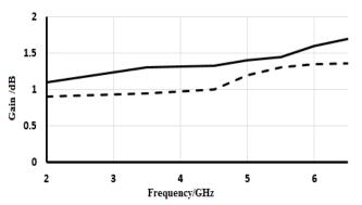
Fig.13: Simulated and Measured Gain of the Fractal MIMO Antenna of Port1
