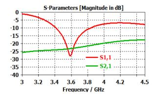
Fig. 5: S-Parameters of the Sierpinski MIMO antenna
