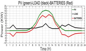
Fig.9. Graph of the Power (PV, LOAD, BATT)
