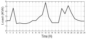
Fig.6. Graph of the daily consumption of the telecom site and electric vehicles
