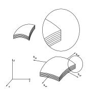
Fig.1. Multilayer three-four-angle shell finite element
