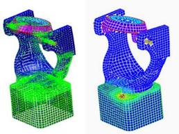
Fig. 2. Distribution of displacements and stresses in the stand when a load is applied to locking device
