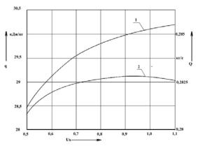
Fig.3. Dependences of specific energy consumption (1) and productivity (2) of KDU-2 shredder on voltage for clover hay
