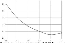
Fig.4. Dependence of mixing irregularity of C-12 feed mixer on voltage  $% \left( {{\Gamma _{\mathrm{s}}} \right)^{2}} \right)$
