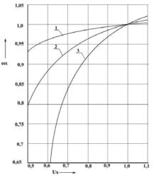
Fig. 7. Change of angular speed from voltage in electric drives of bucket elevator at nominal sliding of the motor: 1-0.02; 2-0.05; 3-0.1
