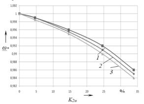
Fig. 8. Dependences of change of angular speed of the electric motor on coefficient of voltage asymmetry on reverse sequence for a drive of working machines with an indicator of mechanical characteristic degree 1 - x = 1, x = 2; 2 - x = 0; 3 - x = -1
