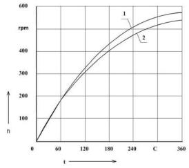
Fig. 5. Acceleration curves of the milk separator COM-3-1000M at nominal (1) and reduced in  $\sqrt{3}$  times voltage (2)
