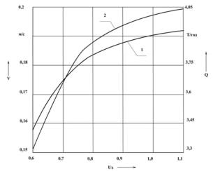
Fig.1. Dependences of speed (1) and productivity (2) of the manure conveyor TSN-2,0B on voltage in relative units
