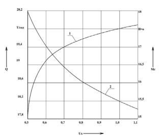
Fig .6. Dependences of productivity (1) and moment of static resistances (2) of noria NZ-20 on voltage.
