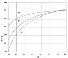
Fig. 2. Dependences of productivity (Q), pressure (H) and power (P) of the centrifugal pump KM8/18 on voltage in relative units
