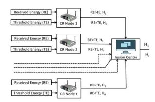
Fig.2. System Model for cooperative spectrum sensing
