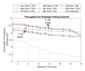
Fig. 5. Attainable throughput for a stand-alone and collaborative CR under Rayleigh channels
