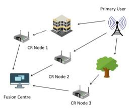
Fig. 1. Illustration of cooperative spectrum sensing scheme
