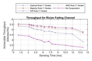
Figure 4. Attainable throughput for a stand-alone and collaborative CR under Rician channels.
