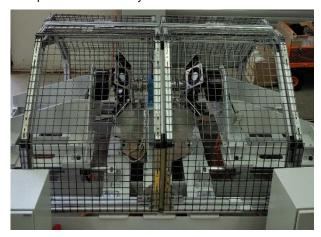
Figure 3 - rotating parts of the test stand enclosed in a cage
