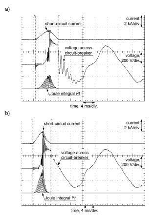
Fig.6. Oscillograms of the real short-circuit current, voltage drop as well as Joule integral (let-through energy) during breaking of current by a circuit-breaker D20, for the value of a prospective short-circuit current: a) 1 kA (5.6 kA<sup>2</sup>s), b) 2 kA (6.5 kA<sup>2</sup>s)
