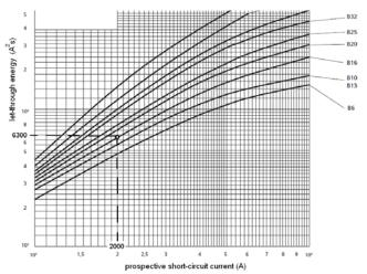
Fig.3. Maximum let-through energy of B-type circuit-breakers declared by the manufacturer [10]; the marked value of the let-through energy (6300  $\mathsf{A}^2s$ ) for a circuit-breaker B16 and a prospective short-circuit current 2 kA
