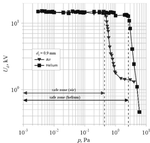
Fig.11. Comparison of safety zones for air-filled and helium-filled vacuum chamber, for contact gap  $d_2 = 0,9$  mm
