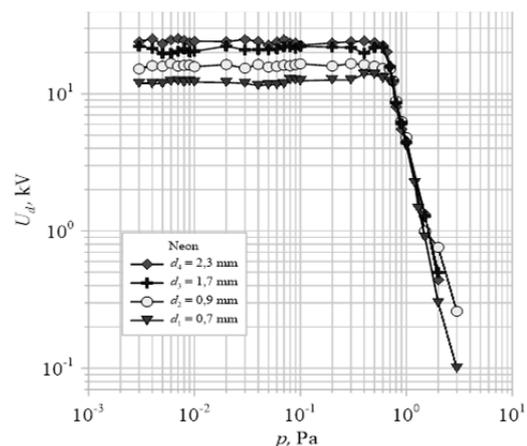
Fig.6. Dependence of the breakdown voltage  $U_d$  as a function of pressure  $p$  for a vacuum chamber filled with neon
