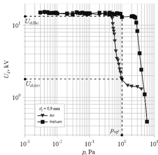
Fig.10. Comparison of the breakdown voltage  $U_d$  as a function of pressure  $p$  for a vacuum chamber filled with air and helium, for the contact gap  $d_2 = 0,9$  mm
