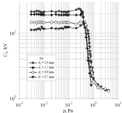
Fig.5. Dependence of the breakdown voltage  $U_d$  as a function of pressure  $p$  for a vacuum chamber filled with air
