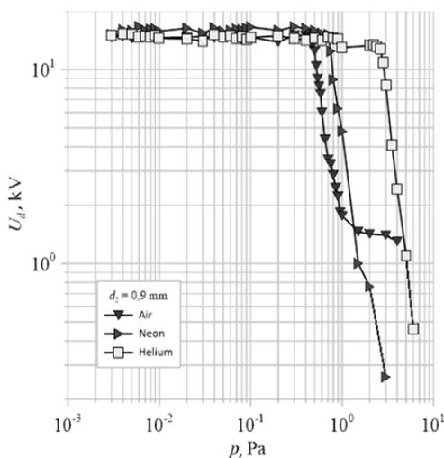
Fig.8. Comparison of the breakdown voltage  $U_d$  as a function of pressure  $p$  for a vacuum chamber filled with air, neon and helium, for a contact gap  $d_2 = 0,9$  mm
