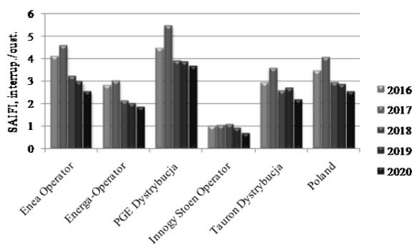
Fig.3. SAIFI from 2016 to 2020 by Distribution System Operators in Poland [2]
