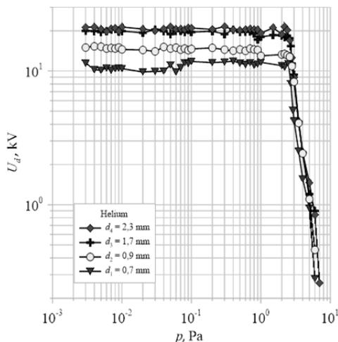
Fig.7. Dependence of the breakdown voltage  $U_d$  as a function of pressure  $p$  for a vacuum chamber filled with helium
