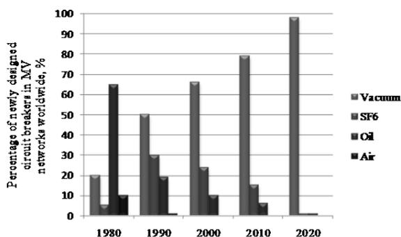
Fig.1. Circuit-breakers in MV networks from 1980 to 2020 by applied insulation medium [1]
