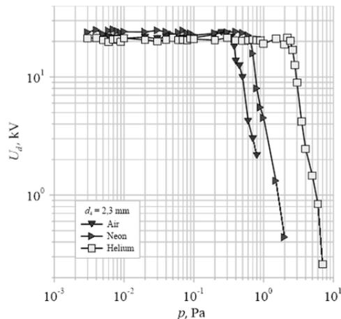
Fig.9. Comparison of the breakdown voltage  $U_d$  as a function of pressure  $p$  for a vacuum chamber filled with air, neon and helium, for a contact gap  $d_4 = 2,3$  mm
