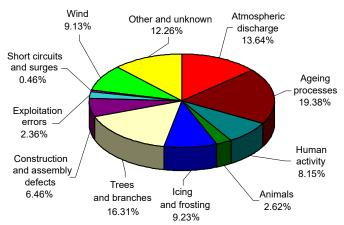
Fig. 2. Percentage share of the causes of overhead MV line failures
