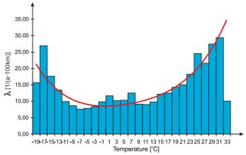
Fig. 3. Dependency of the failure intensity of overhead MV power lines on ambient temperature
