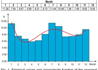
Fig. 1. Empirical values and approximate function of the seasonal variance in the frequency of failures of overhead MV lines
