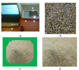
Fig.1. Options for obtaining a computer digital image: a - scanning; b, d - converted photosection image after scanning and photography, respectively; c - digital photography on a green background; 1 - transparent baking sheet; 2 - initial mixture; 3 - scanner; 4 - computer.
