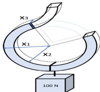
Fig.1. Schematic view of the crane hook design problem
