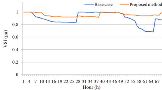
Fig. 7. VSI for base case and Reconfiguration with placement of DG and capacitor in 69-bus test system
