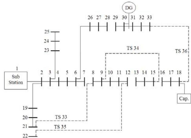
Fig. 1. Network Reconfiguration by installation of DGs and Capacitor in 33-node test system
