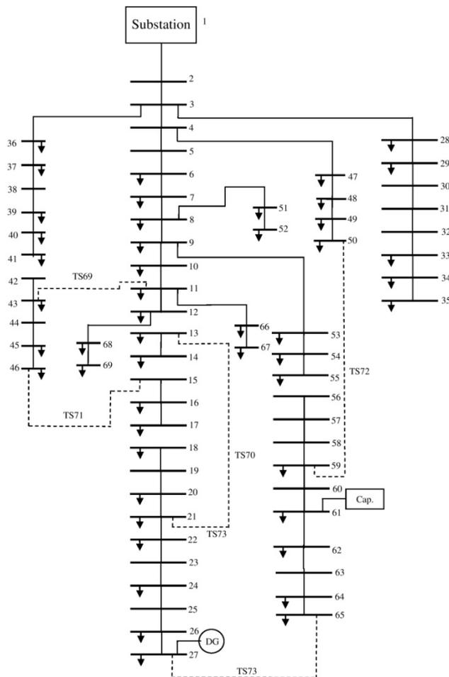
Fig. 5. Network Reconfiguration with placement of DG and Capacitor in 69 node test system
