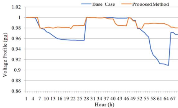
Fig. 6. Voltage profile for base case and Reconfiguration with placement of DG and capacitor in 69-bus test system
