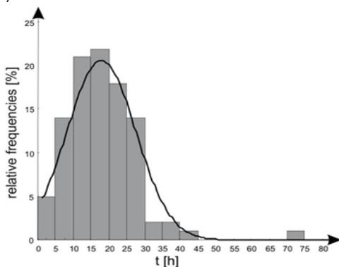
Fig. 5. Empirical distribution determined by simulation for 100 generated values according to normal (bar chart) and theoretical (solid line) distribution
