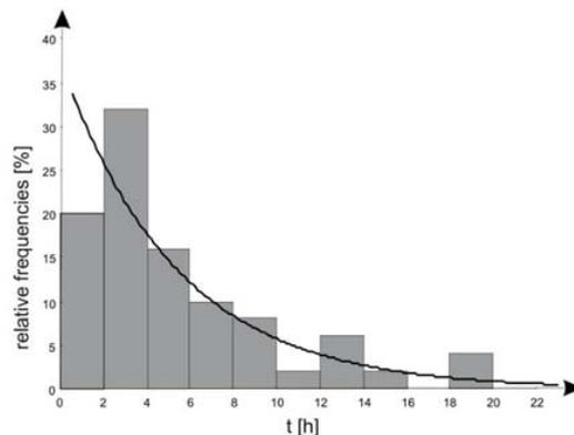
Fig. 1. Empirical distribution determined by simulation for 50 generated values according to exponential (bar chart) and theoretical (solid line) distribution
