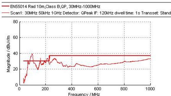
Fig.10. Result of the measurement of radiated emission by printer No. 2 on standby, at a distance of 10 m
