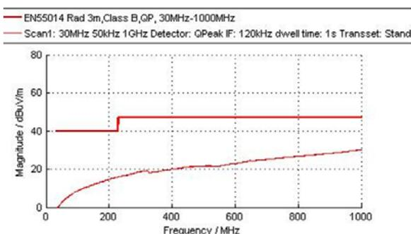
Fig.3. Result of the measurement of the radiation background emission at a distance of 3 m
