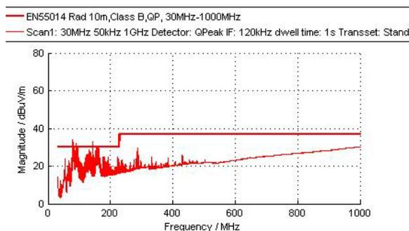
Fig.6. Result of the measurement of radiated emission by printer No. 1 on standby, at a distance of 10 m
