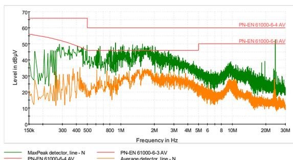
Fig.16. Conducted disturbance measurement results, line N, Prusa i3 MK3S+ printer
