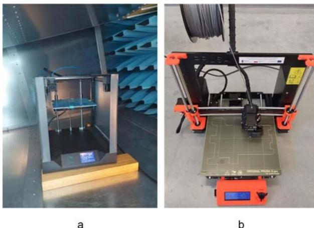
Fig.2. The Sapphire Pro printer (No. 1) placed in the GTEM 1000 cell (a) and a view of the Prusa i3 MK3S+ 3D printer (No. 2) (b)
