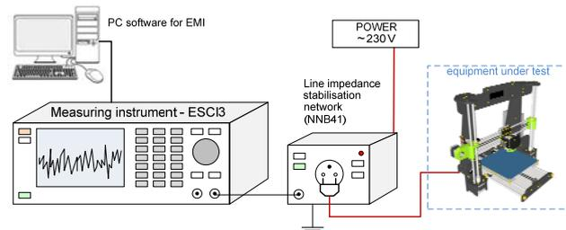
Fig.13. Structure of the measuring system for conducted disturbance analysis
