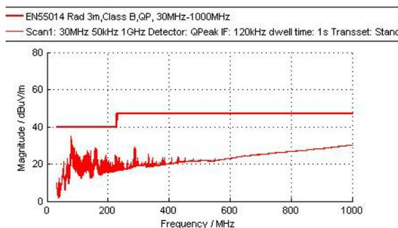
Fig.5. Result of the measurement of radiated emission by printer No. 1 on standby, at a distance of 3 m
