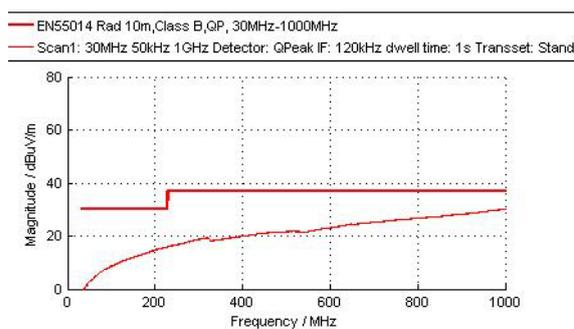
Fig.4. Result of the measurement of the radiation background emission at a distance of 10 m
