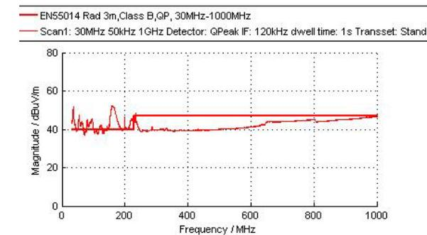
Fig.7. Result of the measurement of radiated emission by printer No. 1, during printing, at a distance of 3 m
