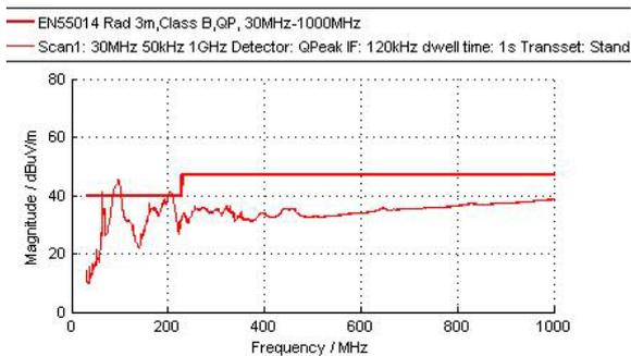
Fig.9. Result of the measurement of radiated emission by printer No. 2 on standby, at a distance of 3 m
