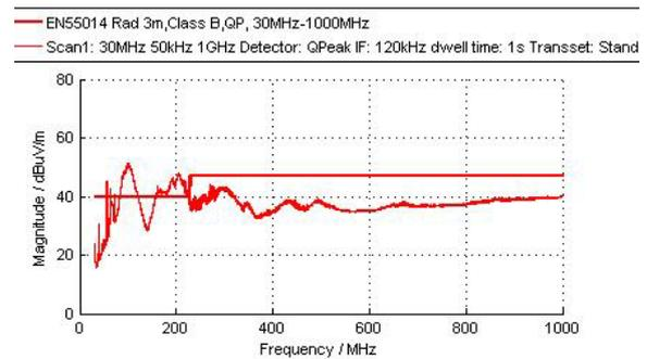
Fig.11. Result of the measurement of radiated emission by printer No. 2, during printing, at a distance of 3 m
