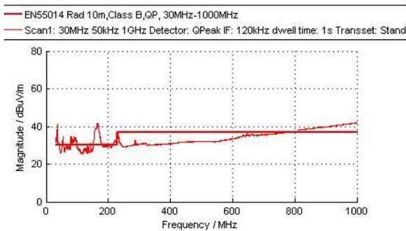
Fig.8. Result of the measurement of radiated emission by printer No. 1, during printing, at a distance of 10 m
