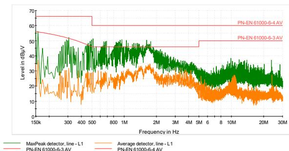
Fig.15. Conducted disturbance measurement results, line L1, Prusa i3 MK3S+ printer
