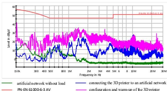
Fig.14. Identification of the conducted disturbance level at the 3D printer site, measurement of the emission level of the artificial network and the 3D printer connected to it
