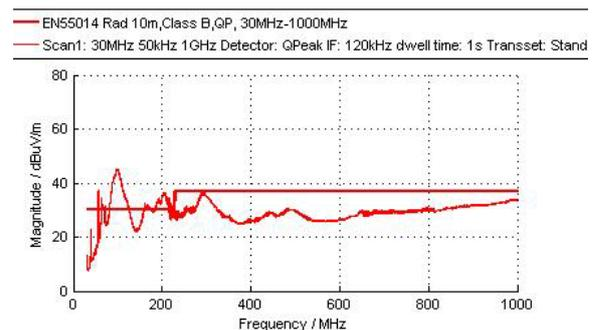
Fig.12. Result of the measurement of radiated emission by printer No. 2, during printing, at a distance of 10 m
