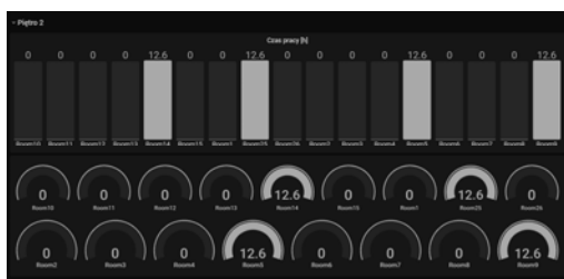
Fig.9. Work time register created with the help of Grafana software
