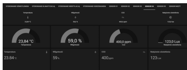
Fig.5. View of the service presenting data from the selected sensor unit
