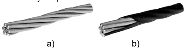
Fig. 1. General type of prototypes: a) AC-50/8 wire; b) modified wire
