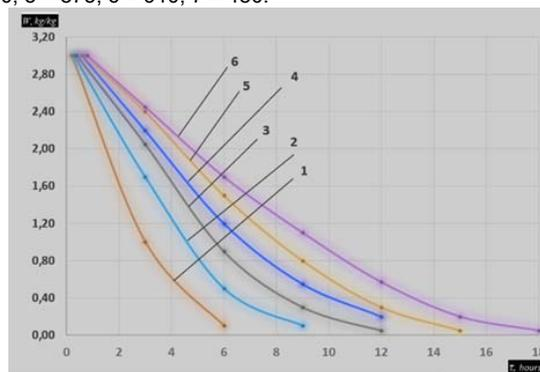
Fig. 4. Kinetics of drying from the proportion of specific load of the material  $P_{sh}$  ( $\text{kg} / \text{m}^2$ ) at  $\Delta d = 10,1\text{ gr}_{\text{moist.}}/\text{kg.sp.}$ ,  $G_n = 500\text{ m}^3 / \text{h}$ : 1 – 13.8; 2 – 21.6; 3 – 28.9; 4 – 36.1; 5 – 43.5; 6 – 50.5.
