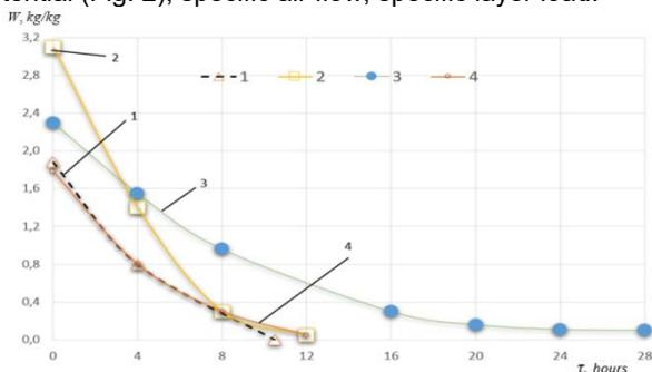
Fig. 2. Kinetics of drying from the initial drying potential  $\Delta d$  ( $g.\text{moist.}/\text{kg.sp.}$ ) at  $P_{sh} = 21.0\text{ kg} / \text{m}^2$ ;  $G_n = 500\text{ m}^3 / \text{year}$ : 1 – 10.2; 2 – 4.5; 3 – 6.7; 4 – 10.0.
