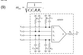
Fig.3. Parasitic elements of AD830
