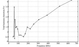
Fig.9. Total harmonic distortion of sinusoidal signals
