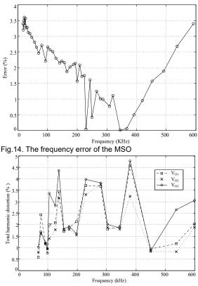
Fig.15. The total harmonic distortion percentage of the MSO
