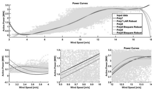
Fig. 7. Model comparison obtained with one variable polynomial
