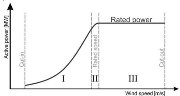
Fig. 1. Wind turbine perfect power curve
