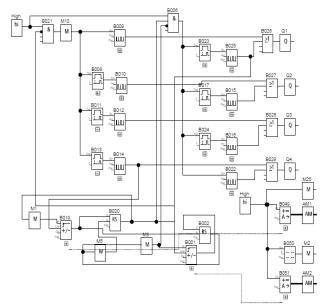
Fig. 3. Control program for the stepper motors using One-phase ON stepping excitation method  $% \left( {{{\rm{C}}_{\rm{B}}}} \right)$
