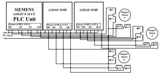
Fig. 1. PLC based stepper motors control connection diagram
