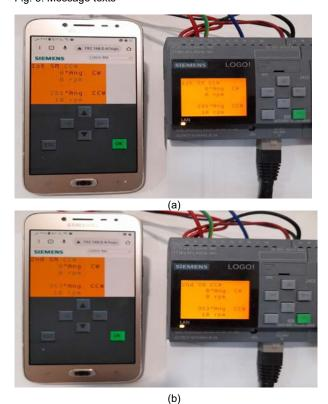
Fig. 6. Message texts are displayed on both the PLC display unit and smart phone.
